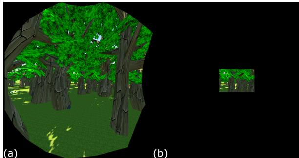
Fig. 2: (a) View of the VE in the left eye with no FOV modification (110°). (b) View of the VE in the left eye with a 40° FOV restrictor.
