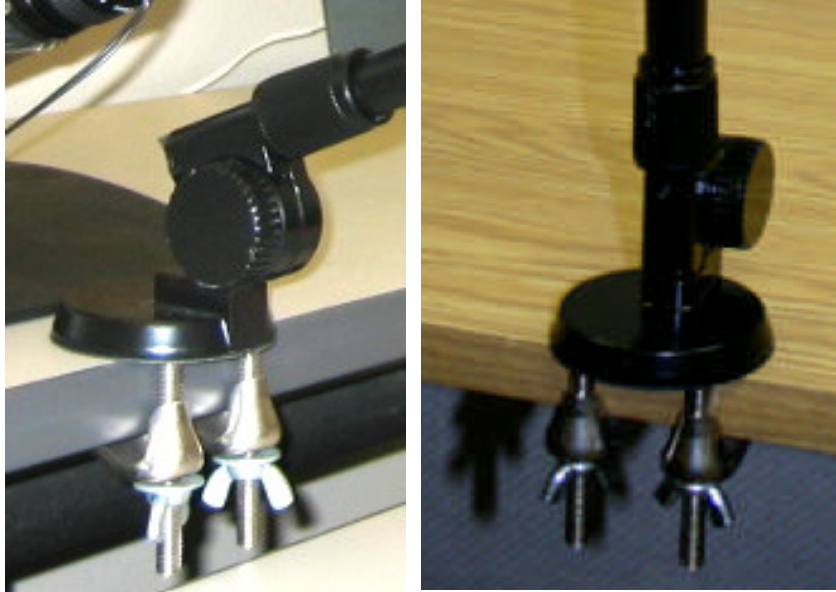
Figure 3. Note how our use of the base of the chinrest (left) is reversed from how it is intended to be used (right). This is made possible by extra threaded holes on the bottom of the base. (Image on the right from richmondproducts.com)
